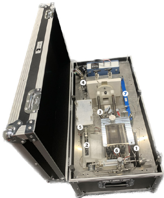
Figure 2. Setup of the atmospheric methane sampling device. The whole system fits well into a box of 80 × 40 × 30 cm. It runs either on 115/230 V AC or 48 V DC provided by a battery pack. Major parts of the system are (1) the Nafion dryer (mostly hidden underneath), (2) pumps (partially hidden), (3) CO 2 trap, (4) flow controller, (5) furnace for CH 4 combustion, (6) sample trap with Peltier coolers, and (7) CO 2 sensor.
