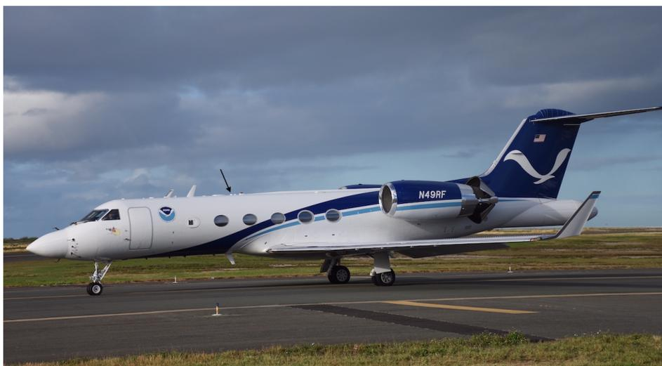
**Figure B1.** The NOAA G-IV aircraft (registration #N49RF) on the taxiway of Honolulu Daniel K. Inouye International Airport (HNL) before departure for an AR Recon flight on 31 January 2021. The black arrow marks the location of the science GNSS antenna mounted on top of the fuselage.
