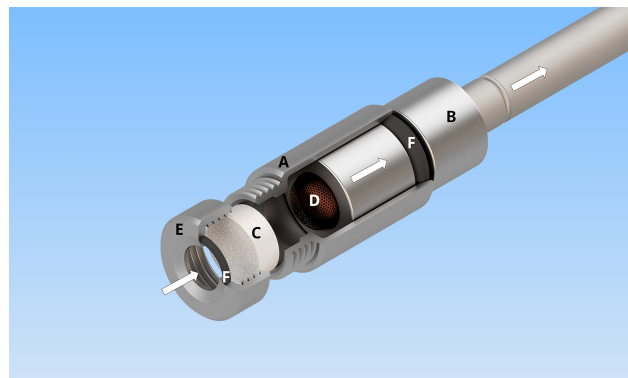
Figure 1. Schematic layout of the ozone scrubber. The scrubber housing (a) was designed to fit on a commonly used diffusion-locking cap (b). Sample airflows from the left to the right, passing both a loaded glass filter as an ozone scrubber (c) and copper wool (d). A screw cap (e) facilitates the quick and easy exchange of the filter. Two O-rings (f), located between the screw cap and the filter and between the housing and the diffusion-locking cap, prevent sampled air from bypassing the filter. Arrows indicate the direction of the airflow through the ozone filter.
