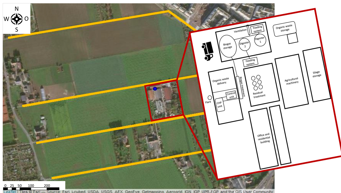
Figure 1. Map of the biogas plant site near Heidelberg, with the emission source location selected for implementing the GPM marked as a blue dot. A zoomed-in schematic of the plant shows the locations of the digesters, biogas storage, and CHP unit. Roads accessible for driving are marked in yellow. The map was created using Leaflet for R.
