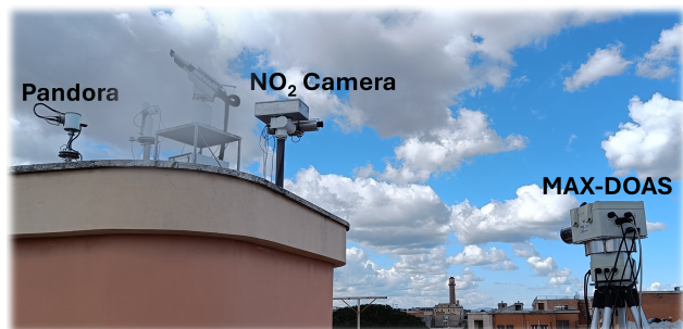
Figure 2. The NO 2 camera and the two reference instruments installed for the campaign at the BAQUNIN-APL supersite.
