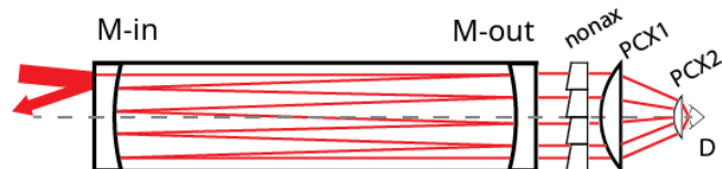
Figure 6. Schematic of the ChiWIS cell and detection optics with the NonAx component included. The NonAx optic is placed between the cavity output mirror and PCX1, where the output rays are nearly paraxial, and refracts out most of the skewness in those rays before they are focused down to the optical axis and onto the detector. Figure adapted from (Clouser et al., 2018).
