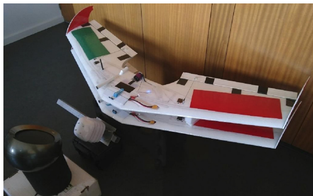
Figure A1. Setup of the 24 h intercomparison measurement of the temperature and humidity sensors (SHT75) installed inside the white tube of each UAV and a reference sensor (SHT21, inside the radiation shield) placed in front of both UAVs. A fan ensured continuous air flow. The experiment was conducted from 4 to 5 June 2021.
