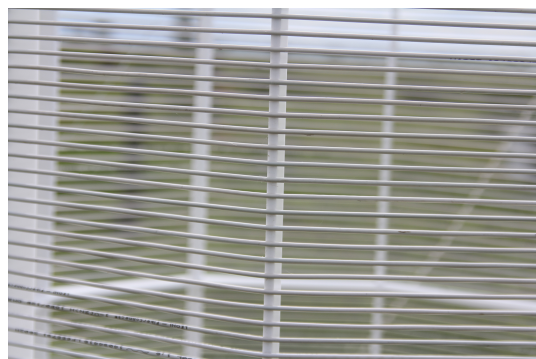
Figure 2. Close up of the coil. The fiber optic cable is kept firmly in place due to the notches on the ribs. Fiber position and spacing is accurately defined as can be seen in the image. The distance between the fibers is very consistent, meaning that its position is precisely defined.
