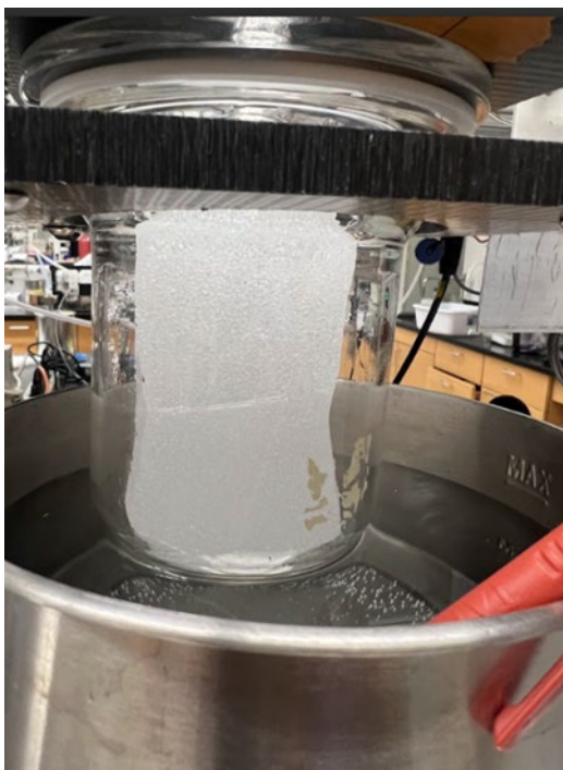
Figure S4. Extraction line in the laboratory. a) extraction line connected to working standards for system calibration, with empty glass flasks, b) glass chambers sealed with ice core samples prior to melting c) close-up of glass flask containing an ice core sample about to be immersed in warm water. The plastic outer ring is visible at the top of the flange, d) top view of the glass chamber. The PTFE inner ring is visible. Used with permission of Miranda H. Miranda.
