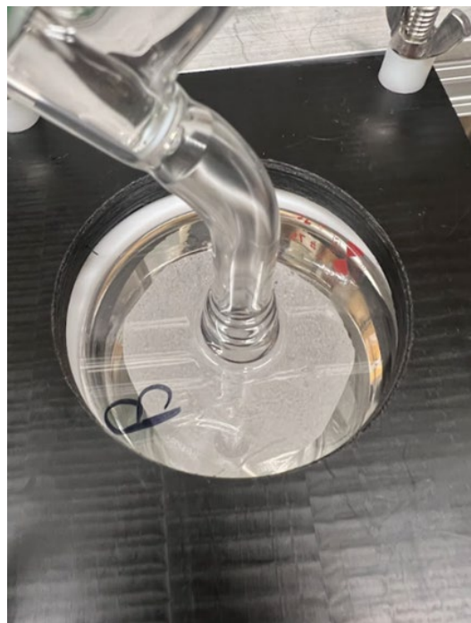
Figure S4. Extraction line in the laboratory. a) extraction line connected to working standards for system calibration, with empty glass flasks, b) glass chambers sealed with ice core samples prior to melting c) close-up of glass flask containing an ice core sample about to be immersed in warm water. The plastic outer ring is visible at the top of the flange, d) top view of the glass chamber. The PTFE inner ring is visible. Used with permission of Miranda H. Miranda.
