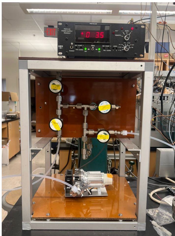
Figure S5. Image of the dilution system showing bellows valves and pump. The Baratron vacuum transducer is mounted behind the panel. Used with permission of Miranda H. Miranda.
