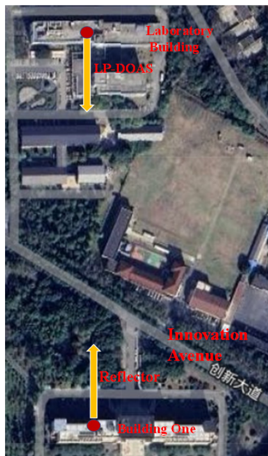
Figure 14. LP-DOAS telescope and reflector position (optical path of 700 m, from © Google Maps).
