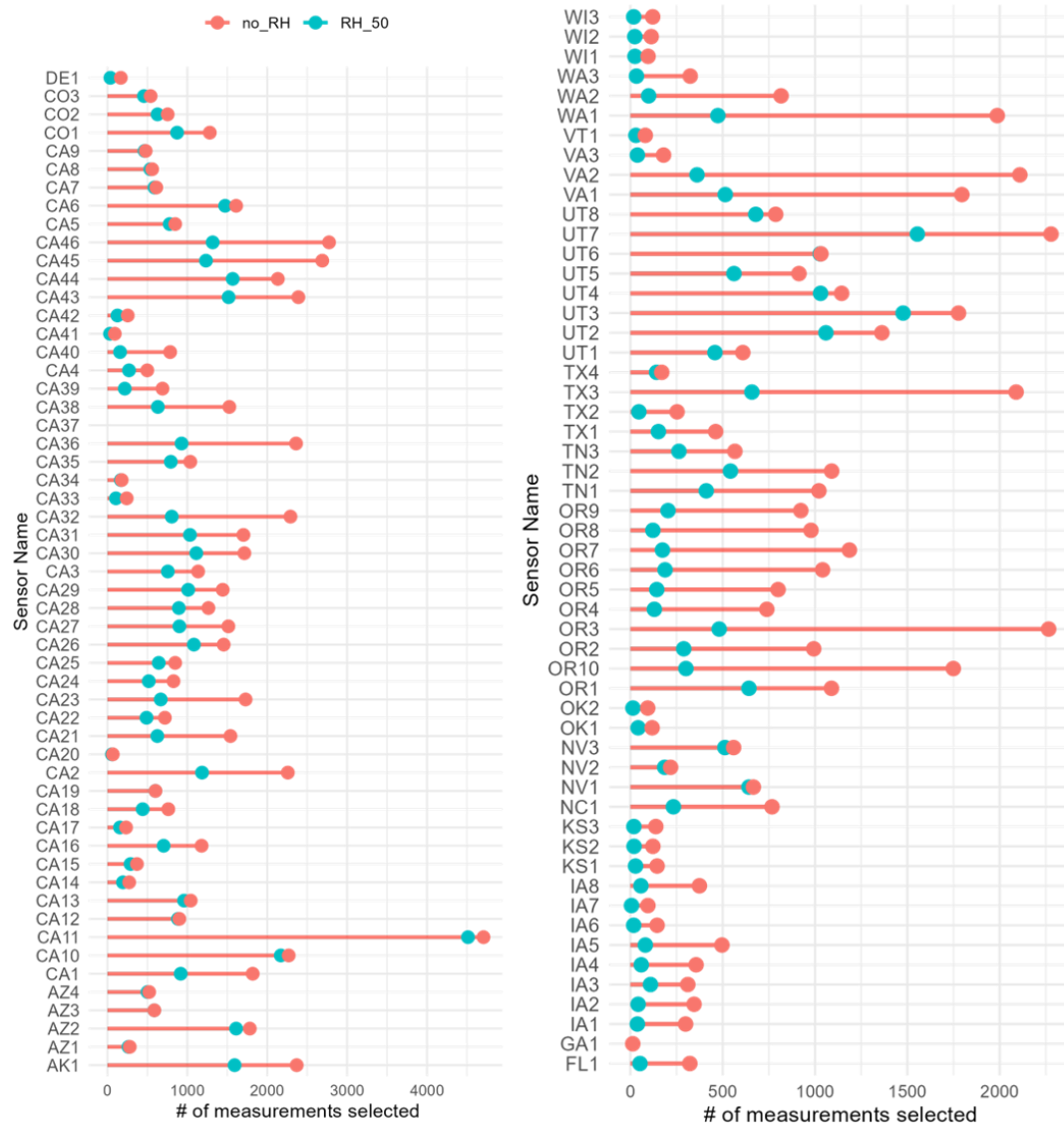
Figure S15: The number of measurements identified as potential dust-dominated PM measurements for the real-time approach when using a RH cutoff of 50% vs. no RH cutoff. For all sensors, using no RH cutoff resulted in the selection of more measurements. The sensor information corresponding to the Sensor Name can be found in Tables S1, S2, and S3.
