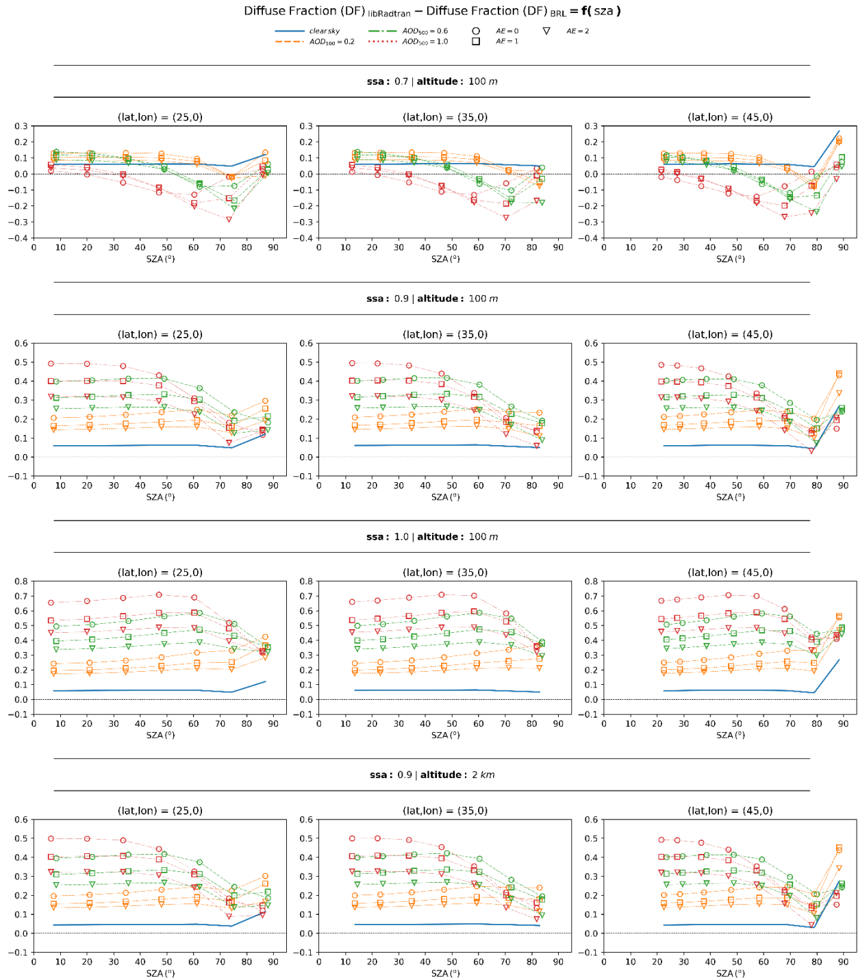
Figure S1. Difference between the diffuse fraction derived directly from the computations of DHI and GHI using libRadtran and the one estimated by applying BRL to the libRadtran-computed GHI for surface albedo 0.8
