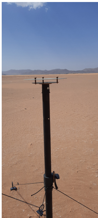
Figure 7. Flat-plate sampler (FPS) used in the J-WADI campaign, adapted from Ott and Peters (2008). Positioned 10 m from the rotating mast, it consists of two brass plates at a distance of 16 mm and a circular substrate (diameter = 25 mm) in the center of the bottom plate.
