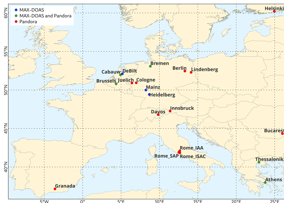
Figure 2. Map of FRM4DOAS MAX-DOAS and PGN Pandora sites used for validating the TROPOMI NO 2 product.
