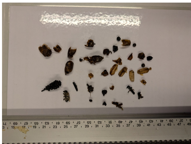
Figure 6. Detritus found in Davis VP2 tipping bucket rain gauge after 7 years of operation. For scale a ruler (cm) is shown along the bottom.
