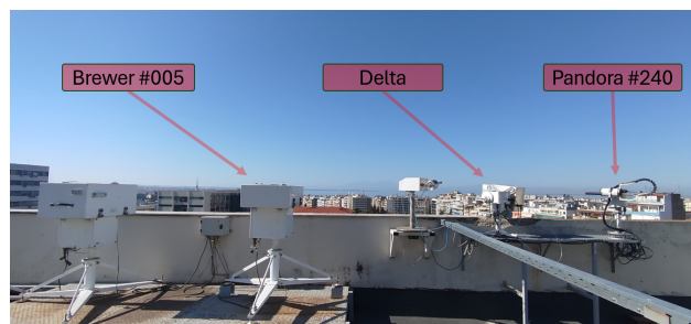
Figure 1. The measurement site of LAP.AUTH and the three collocated ground-based instruments used in this study: Brewer spectrophotometer #005 (left), Delta UV-VIS DOAS system (centre), and Pandora #240 (right).
