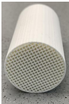
Figure S1 Photograph of the ceramic honeycomb body ( \text{\O} 25,4 \times 50\text{mm} ) used as substrate for \text{Na}_2\text{SO}_3 coating in this study.
