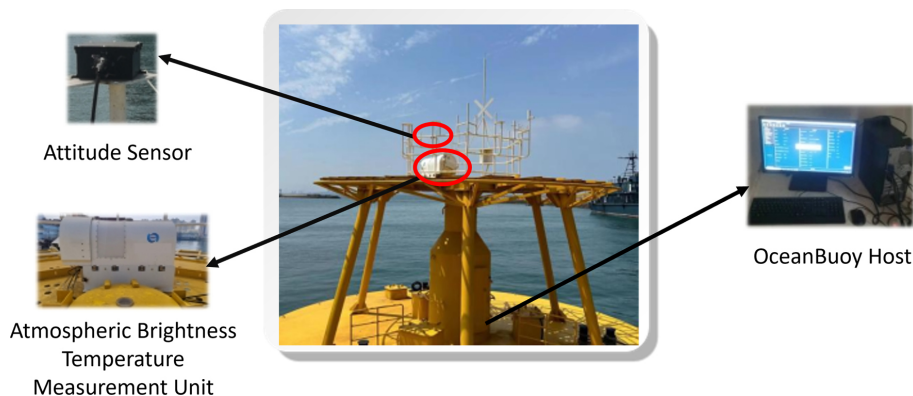
Figure 4. Schematic of the sea trial experimental setup on the 10 m diameter buoy platform. Key components include: the attitude sensor (top left) for monitoring platform roll and pitch; the QFW-6000 atmospheric brightness temperature measurement unit (bottom left) installed on the upper deck; and the OceanBuoy Host (right) for data aggregation and transmission. The red circles in the central photograph indicate the mounting positions of the sensors on the buoy structure.
