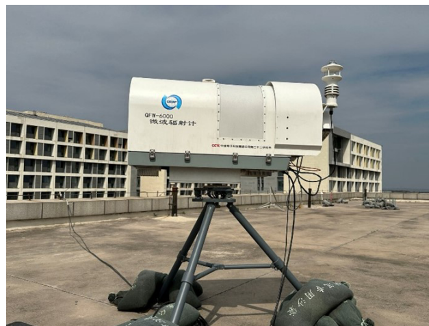
Figure 1. The QFW-6000 microwave radiometric profiler developed by the CETC No.22 Research Institute was deployed for the experiment. The instrument features a K-band and V-band receiver for profiling tropospheric temperature and humidity.
