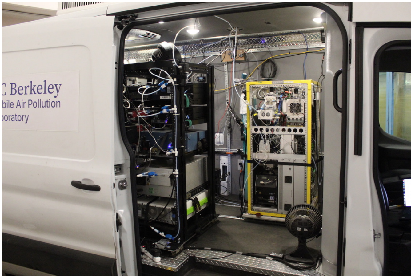
Figure S1 Side on view of the CalMAPLab through the passenger cargo door. On the left is the gas phase rack containing the Aeris \text{CH}_4/\text{C}_2\text{H}_6 , Aeris \text{CO}/\text{N}_2\text{O} , 2BTech \text{O}_3 , CAPS \text{NO}_2 and EcoPhysics \text{NO}_x and on the right is the Vocus PTR-ToF-MS in the yellow rack. Sample lines can be seen entering through the roof inlet plates and distributed to the different instruments.
