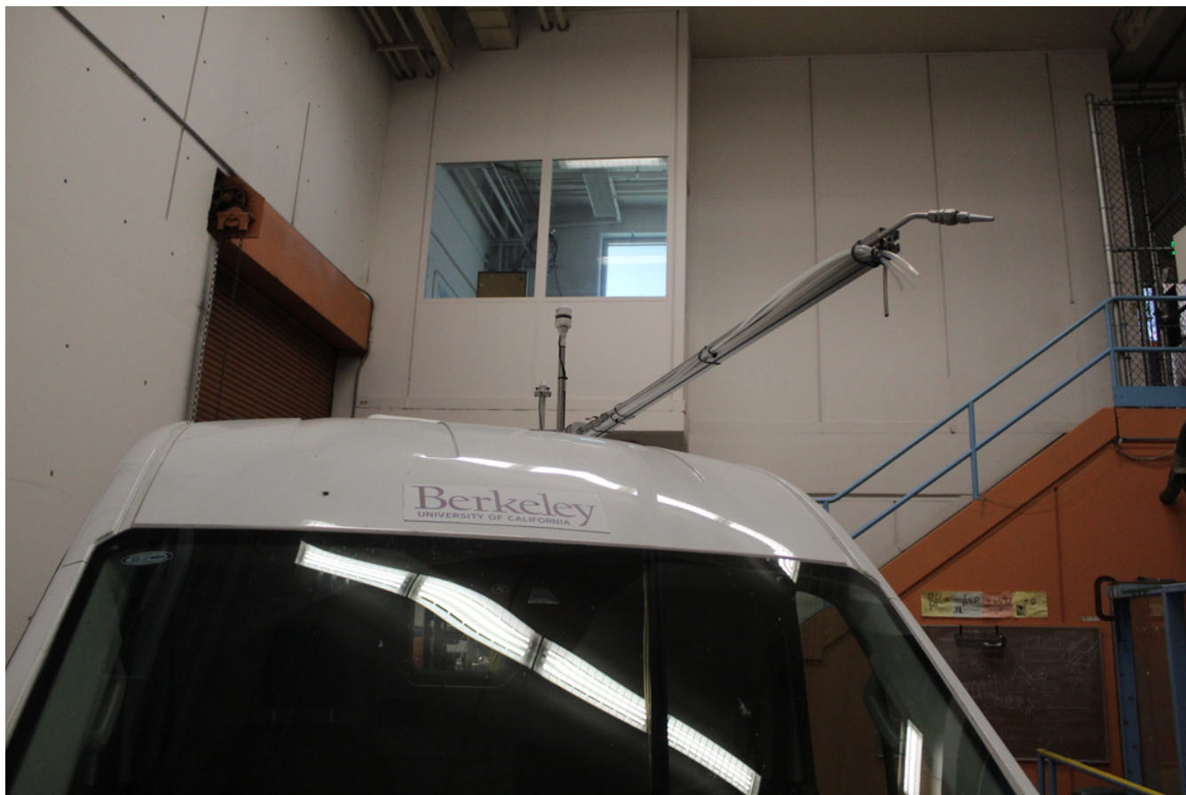
Figure S3: Front-on view of the CalMAPLab in its indoor parking space featuring the gas and particle phase inlet lines mounted to an extruded aluminium rail. Also visible are the Airmar WX200 weather station and MetOne pyranometer.
