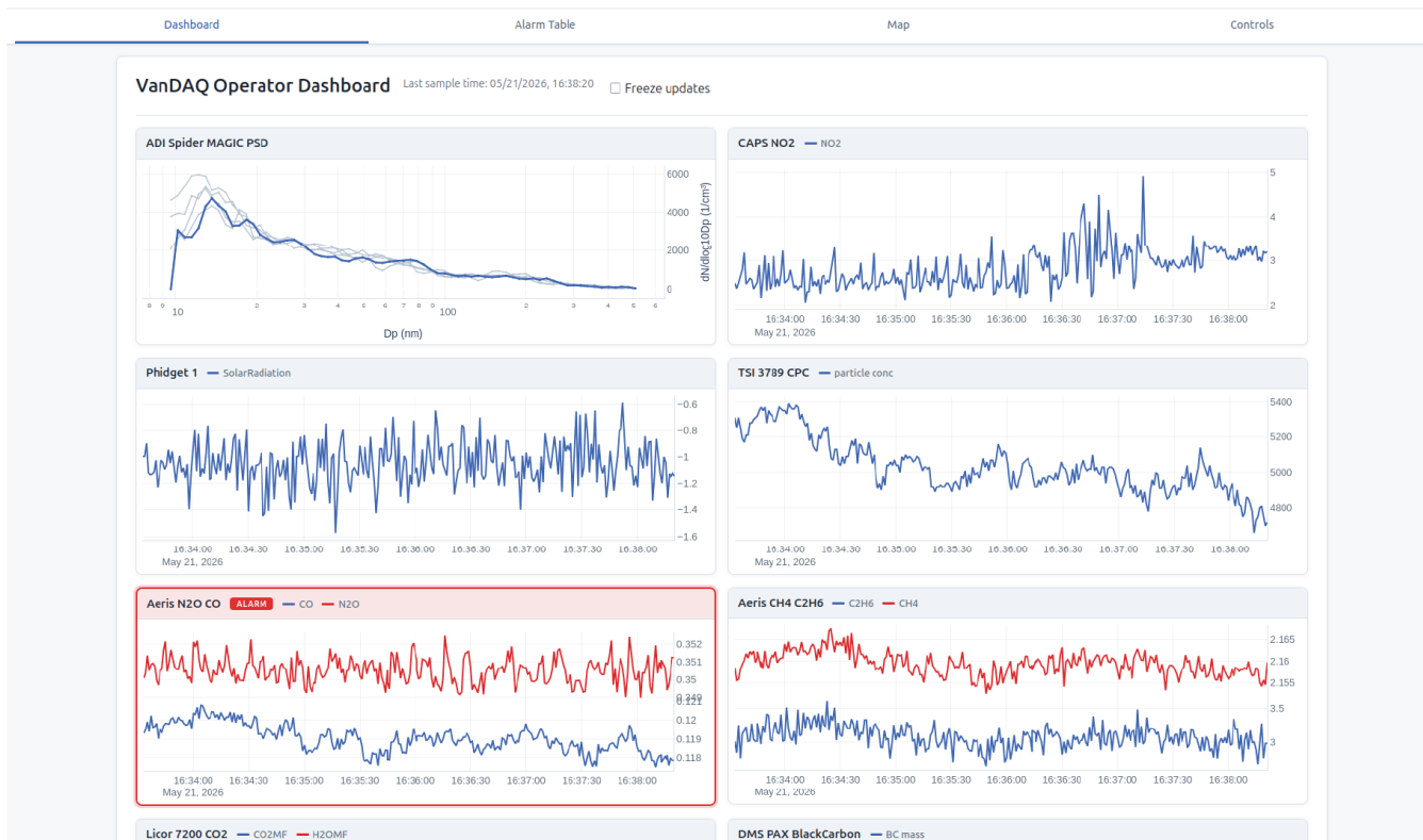
Figure S5: VanDAQ time series dashboard for key measured species by instrument. Individual panels can be configured to show multiple species on different axis (e.g. Aeris instruments). Standard operations display the last 5-minutes of data. Should a measured parameter be out of range (e.g. Aeris CO/N 2 O), that instrument flashes red to alert the operator.
