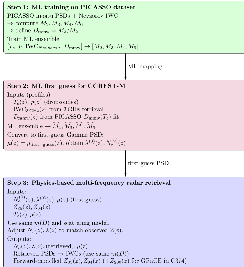
Figure 6. A schematic overview of the retrieval framework. Step 1: an ensemble ML model is trained on the PICASSO dataset using in-situ PSDs and the Nevzorov IWC to compute the PSD moments M_2, M_3, M_4 and M_6 and the mean mass-weighted diameter D_{mmw} = M_3/M_2 . Step 2: for each CCREST-M case, profiles of T_c, p , 3 GHz-retrieved IWC and D_{mmw}(T_c) are passed through the ML ensemble to predict the moments, which are converted into first-guess gamma PSD parameters, with \mu(z) = \mu_{\text{first-guess}}(z) , where z is the altitude, and corresponding \lambda^{(0)}(z) and N_o^{(0)}(z) . Step 3: a physics-based multi-frequency radar retrieval adjusts N_o(z) and \lambda(z) using the same m(D) and scattering model so that simulated reflectivities Z_{35}(z) and Z_{94}(z) match the observations, yielding retrieved PSD parameters, PSDs and estimated IWCs, and forward-modelled reflectivities.
