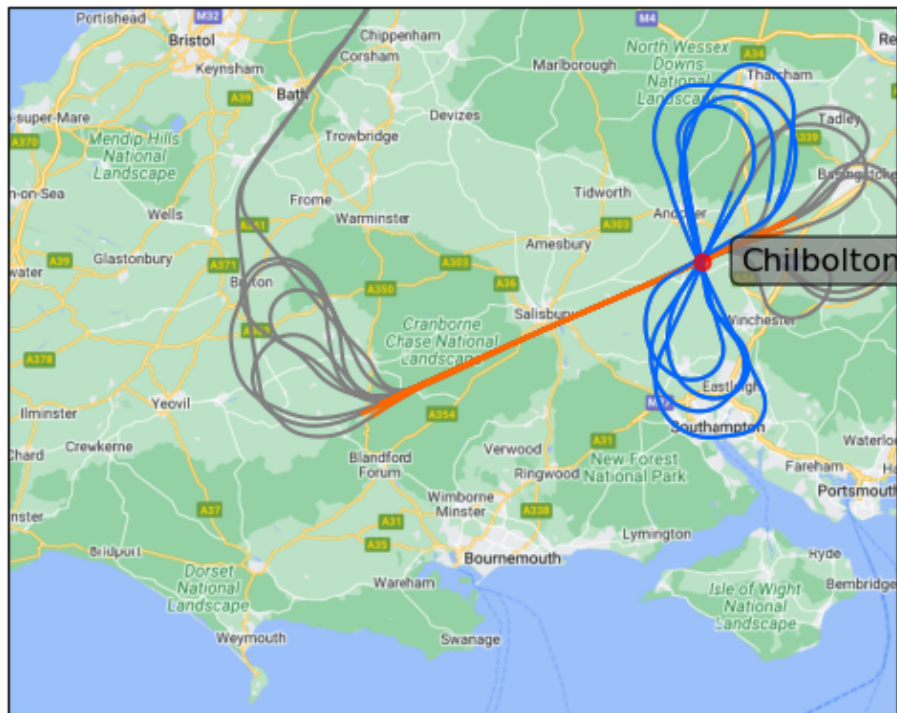
Figure 1. A typical CCREST-M flight track (shown as the grey, orange and blue colours) towards and over the Chilbolton-based triple-frequency radars. The figure-of-eight patterns (blue) were flown over Chilbolton when all the radars were pointing at zenith. The aircraft flew along a specific flight path, known as the Chilbolton radial (orange), which is set at an angle of 246 or 270°. Figure created by Stuart Fox.
