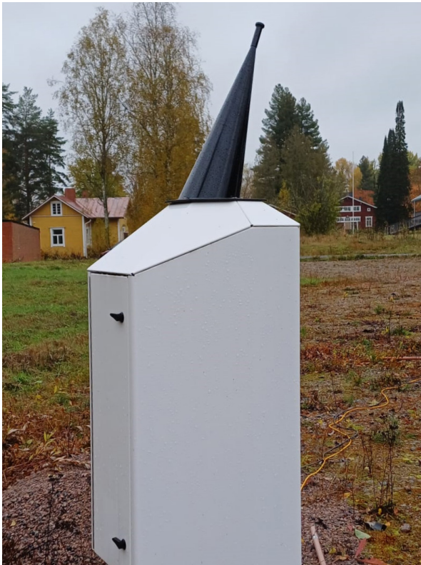
Figure 2. A termination hood (Vaisala CL61TERMHOOD) placed on top of the CL61 in Hyttälä.
