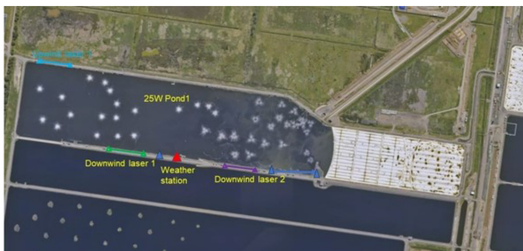
Figure 1. The layout of experimental site with one upwind open-path laser (light blue line with triangles), and two downwind open-path lasers (green and purple for summer campaign, green and blue for winter campaign). The Red triangle shows the weather station location during the summer campaign, while the dark blue triangle shows the weather station location during the winter campaign (Source: Imagery © 2024 Airbus, Map data © Google Earth).
