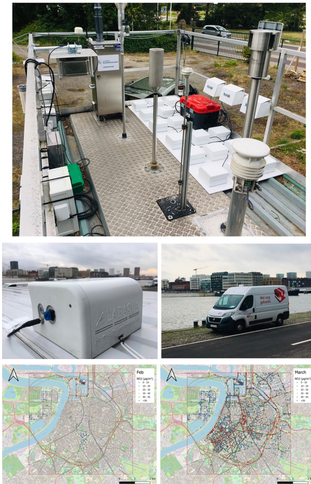
Figure 4. (a) Kunak ® Air Mobile sensor systems co-located at the R817 AQMS; three in fixed shields, 17 in mobile enclosure (upper), details of the Kunak ® Air Mobile sensor system (lower left), and rooftop deployment on a postal van in Antwerp (lower right). (b) maps of monthly collected mobile NO 2 measurements ( \mu\text{g m}^{-3} ) in the city of Antwerp between February and September 2021 (Hofman et al., 2023).
