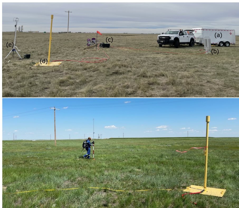
Figure 1. Top panel – Controlled release setup. (a) CNG trailer with tanks. (b) ambient heat exchanger. (c) flow controller. (d) release stack. (e) anemometer. Bottom panel – the pole-based measurement system in operation during a controlled release test on 12 June 2024. The operator carried a \text{CH}_4 sensor in a backpack harness and a long length of hose was run from the sensor's inlet to the end of the pole where air was drawn in. Photo credits Zhenyu Xing and Chris Hugenholtz.
