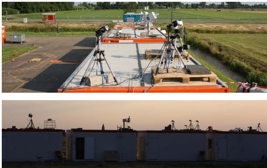
Fig. 3. Some of the roof-top instruments deployed at the campaign site, in views looking to the south (upper) and to the west (lower). Some other instruments were on the ground to the west of these containers; four other instruments were on the tower 370 m to the right of the lower picture; and a further three instruments were at the wind profiler site 160 m to the right of the upper picture.
