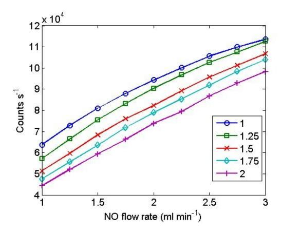
Figure S-3. Instrument response (in counts s<sup>-1</sup>) as a function of nitric oxide flow rate (ml min<sup>-1</sup>), and for different sample flow rates into the reaction chamber (l min<sup>-1</sup>).
