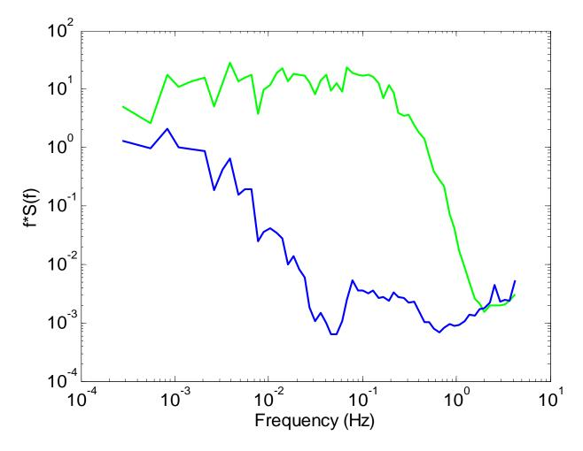
Figure S-5. Power spectrum of the water vapour flux measured with the LI-COR upstream of the Nafion Dryer (green data points) in comparison to the measurements from the LI-COR downstream of the Nafion Dryer (blue data).
