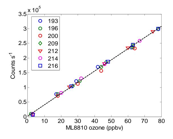
Figure S-4. Calibration of the fast response ozone chemiluminescence instrument (FRCI) with the Monitor Lab (ML) 8810 during the GOMECC-2007 cruise (Day of Year
