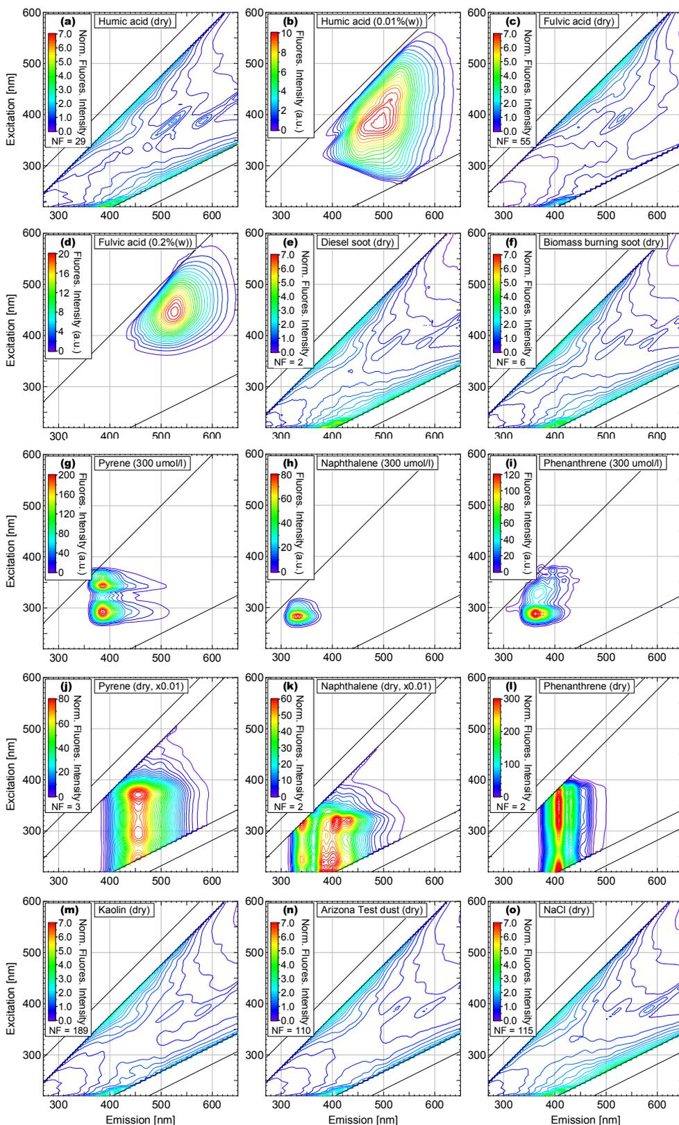
**Fig. 5.** Normalized EEM contour profiles for selected interferences in solid state and/or solution. Intensity color scale has been adjusted to intensity of individual components. All EEMs are normalized as discussed in text (Sect. 3.2). Normalization factor (NF) is reported for each solid-state sample. Lower NF indicates higher fluorescence intensity.
