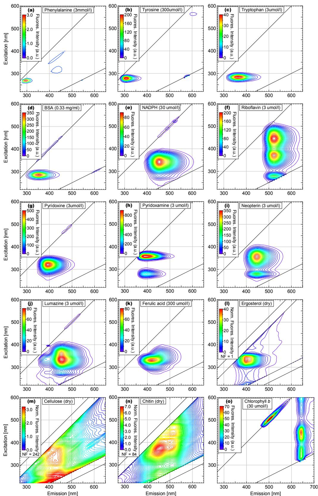
**Fig. 2.** EEM contour profiles for selected pure biological fluorophores in solid or solvated state. Intensity color scale has been adjusted to intensity of individual components. All EEMs are normalized as discussed in text (Sect. 3.2). Normalization factor (NF) is reported for each solid-state sample. Lower NF indicates higher fluorescence intensity. Note change in x-axis scale for chlorophyll-*b*.
