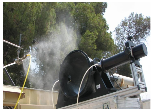
Fig. 20. A controlled experimental setup for validation of the proposed methodology. An artificial cloud was sprayed via an atomizing nozzle and entered the field of view of an accurate particle sizing device (Spraytec). A calibrated spectro-radiometer and a thermal imager were positioned below the passing cloud (not shown), pointing to the zenith.
