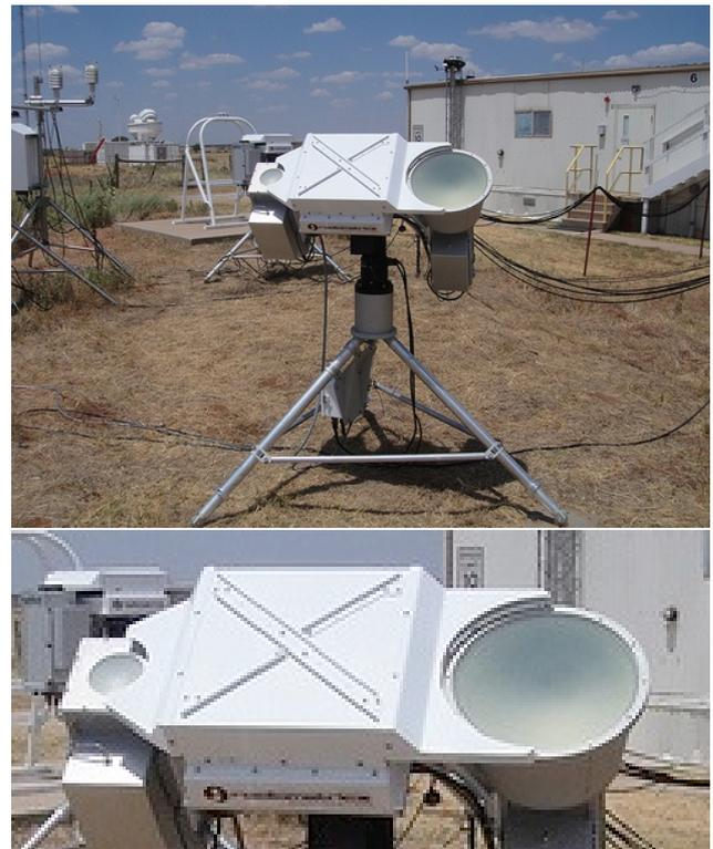
**Fig. 4.** The new ARM 3-channel microwave radiometer (MWR3C) with a view of the rain mitigation system.
