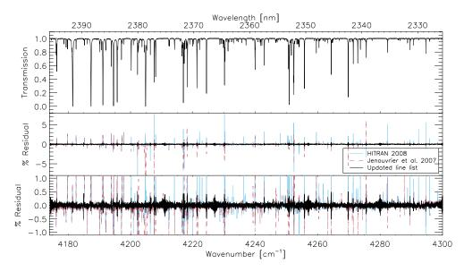
Fig. 1. Top: laboratory spectrum of water vapour for T = 293 K,  $P_{\text{H}_2\text{O}} = 4.04 \text{ hPa}$  and  $P_{\text{air}} = 333.6 \text{ hPa}$ , adopted from Jenouvrier et al. (2007, their run *j*). Middle: fit residuals (measured-modelled times 100) using HITRAN 2008 (blue), the original Jenouvrier et al. (2007) line list (red) and after fitting for the line parameters in this work (black). Bottom: close-up of the middle panel.
