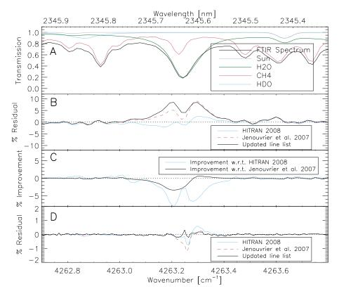
**Fig. 5.** Close-up of Fig. 4 around a line of which the residuals deteriorate. **(A)** Measured normalized transmission. The different colours show the contributions of all the modelled species. **(B)** Residuals. **(C)** Difference between the absolute values of the residuals. **(D)** The corresponding laboratory fit residuals.
