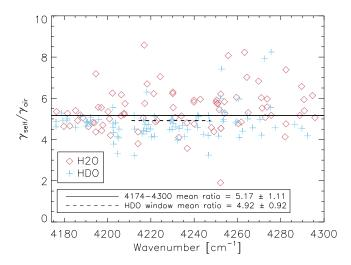
**Fig. 2.** Ratios between the self-broadened and air-broadened half-widths of the original Jenouvrier et al. (2007) spectroscopy. Plotted for the 174 lines with a line intensity stronger than  $10^{-25}$  cm<sup>-1</sup>(molecule cm<sup>-2</sup>)<sup>-1</sup>. The solid and dashed lines indicate the mean ratio for the 4174–4300 cm<sup>-1</sup> and the HDO retrieval window (4212–4248 cm<sup>-1</sup>), respectively.
