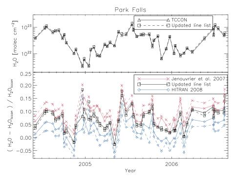
Fig. 7.  $H_2O$  FTS retrieval accuracy for Park Falls. Top: time series of the fitted  $H_2O$  columns using TCCON's GFIT algorithm at  $1.6\,\mu m$ , compared to using our updated line list in the  $4174-4300\,cm^{-1}$  range ( $2.3\,\mu m$ ). Bottom: time series of the relative differences with TCCON for all different line lists. Solid and dashed lines are for the  $4174-4300\,cm^{-1}$  and  $4212-4248\,cm^{-1}$  window, respectively.
