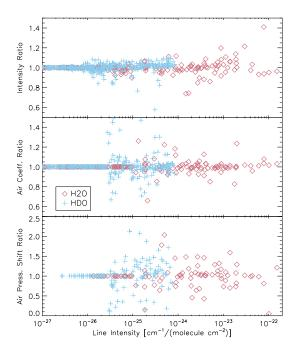
**Fig. 3.** Ratio of the updated line parameters over the original line parameters. Top: line intensities. Middle: air broadening coefficients. Bottom: air pressure shifts.
