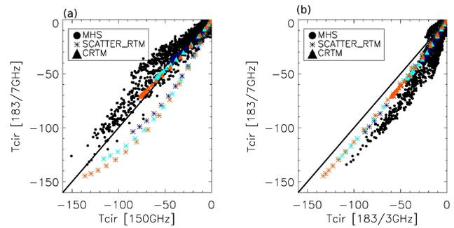
**Figure C1.** Scatter plots of  $T_{\text{cir}}$  relationships between CH#2 and CH#5 (a), and CH#4 and CH#5 (b) from observed  $T_{\text{cir}}$  at MHS nadir view (black dots), simulated  $T_{\text{cir}}$  from CRTM (colored triangles) and from CRM (colored stars). Blue/cyan/red colors represent cloud layer with tops at 10, 12 and 14 km and bottoms at 7.5 km in the simulations.
