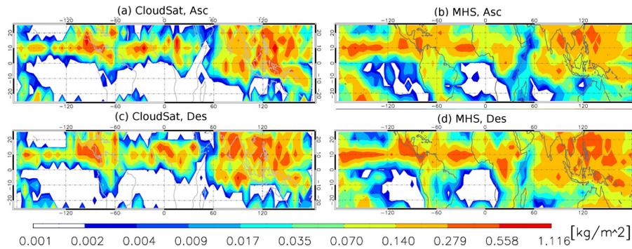
**Figure 8.** Monthly averaged IWP from CloudSat and MHS ascending (a, b) and descending (c, d) orbits during August 2010. MHS IWP is averaged over all views. Data are sampled to  $5^\circ \times 5^\circ$  grid boxes.
