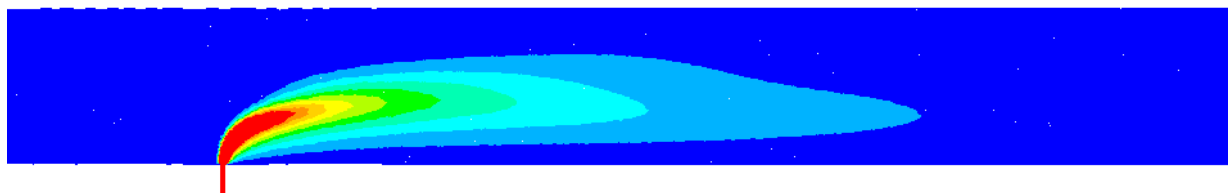
Figure S17a. Contours of ammonia (24 pptv intervals, 240 max). \text{NH}_3 in a sidearm flow of \text{N}_2 (0.05 sLpm) added to the main flow (6sLpm) that is also cooling due to interacting with the wall: from 307 K (incoming at the left) to \sim 298 K (outgoing, right.) NLM is 16 pptv. Note that ammonia is present at ppbv levels in the \text{N}_2 flow (40-100 sccm) exiting the dynamic dilution system, and it mixes down to the tens of pptv levels in the main flow.
