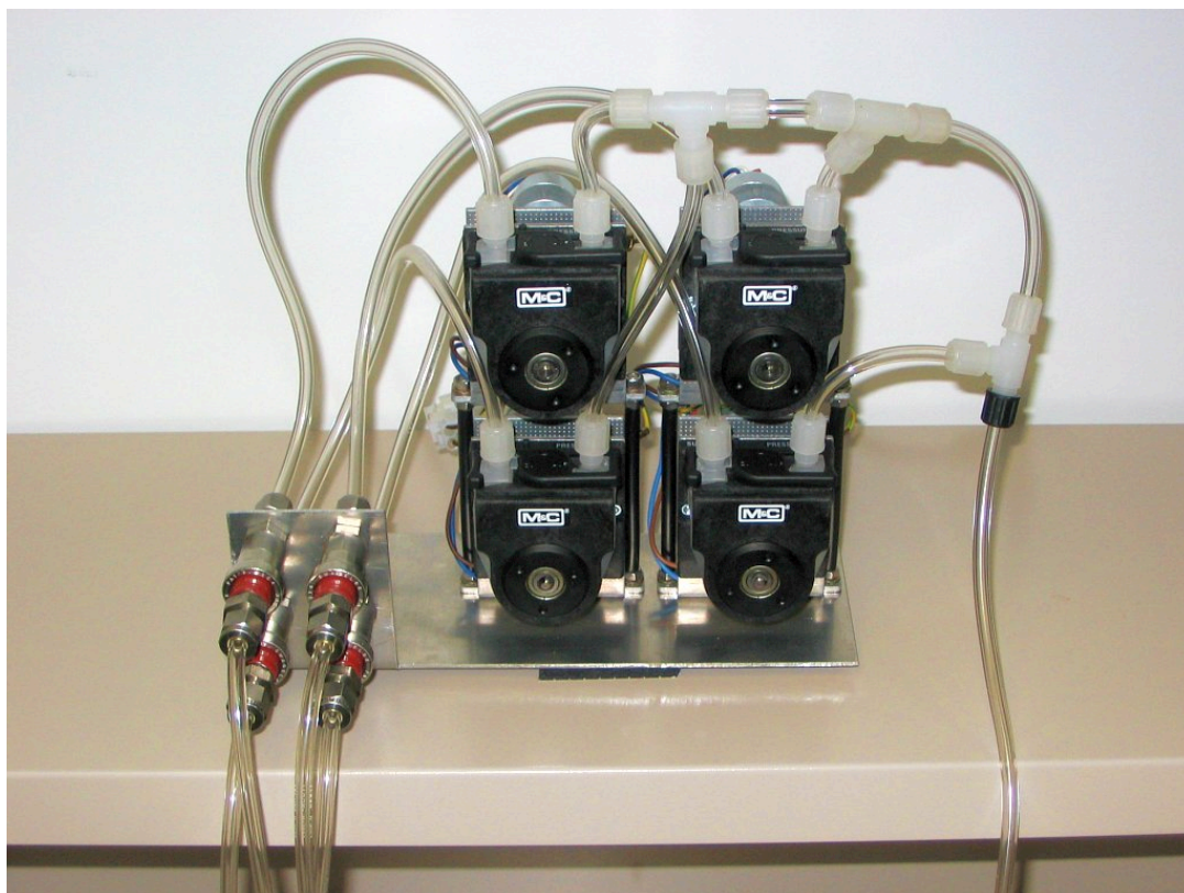
Figure S11. Peristaltic pump assembly for the M&C chiller with modifications to simplify replacement.
