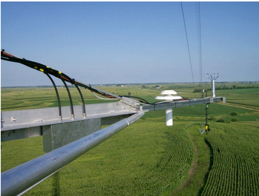
Figure S4. Retractable boom at WBI with three sampling intakes and meteorological sensors. Inlet filters are housed in the aluminum enclosure to which the Synflex tubes are connected. A Yagi antenna that is used to transfer data from the meteorological sensors via radio modem is also visible.
