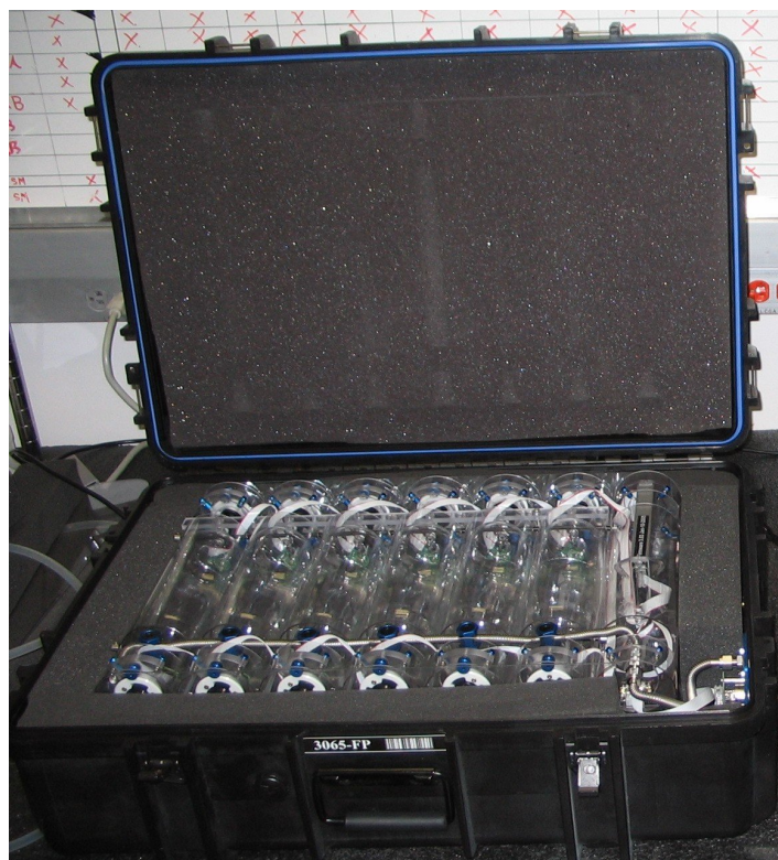
Figure S16. Interior of a Programmable Flask Package (PFP).
