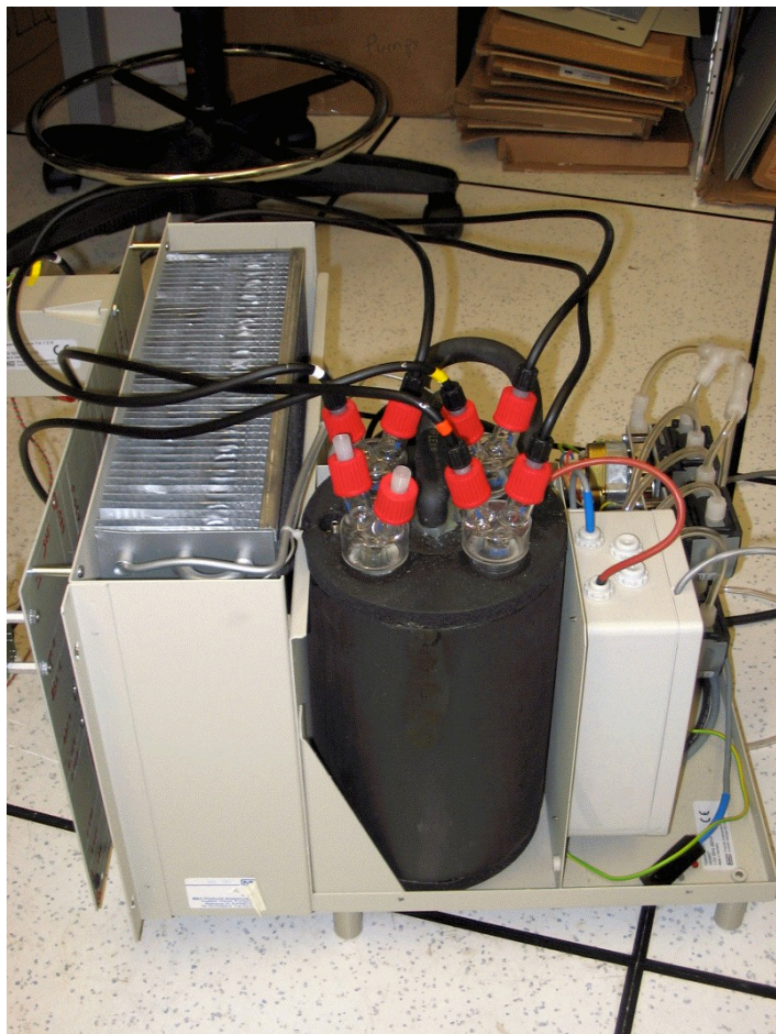
Figure S10. Interior of M&C 4-channel chiller showing the glass condensers.
