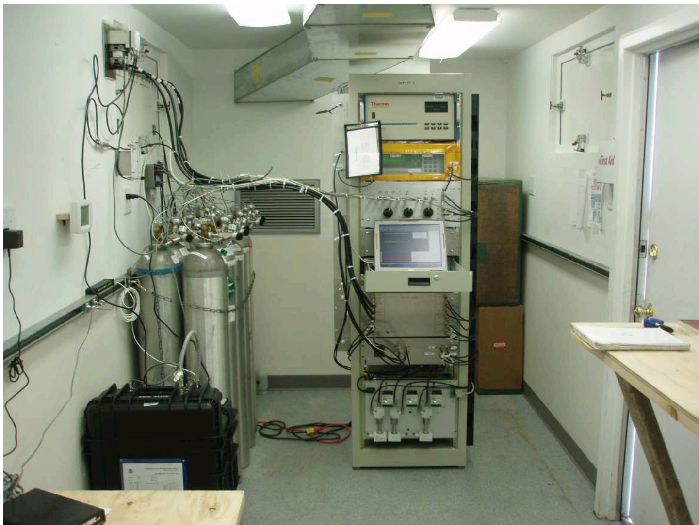
Figure S5. Interior of the sea container laboratory at WBI showing the CO 2 /CO analysis system and calibration gases. The Programmable Flask Package (PFP) is the black plastic suitcase in the foreground. Ducting along the ceiling helps to distribute flow from the HVAC unit. Panels provide access to the outside.
