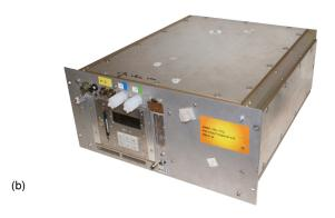
**Fig. 1.** (a) Schematic setup of the airborne FGGA deployed aboard CARIBIC (additional laser for CO<sub>2</sub> measurements not shown). LD: laser diode, FC: fiber collimator, PD: photo detector, PV: proportional valve, p: pressure sensor, T: temperature sensor, FM: flow meter, BV: buffer volume, P: pump, FR: flow restrictor. (b) Photograph of the modified FGGA.
