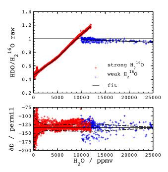
**Figure 3. (a)** Individual calibration measurements on 25 July 2013 pre- and post-flight together with the daily average calibration functions for strong (red) and weak (blue)  $H_2^{16}O$  line fit. (b) Calibration measurements on VSMOW scale corrected for nonlinear response. Dashed lines indicate the  $1\sigma$  confidence band.
