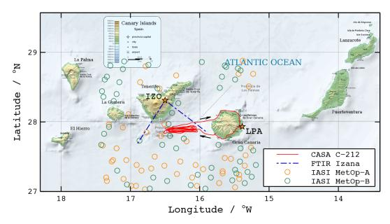
**Figure 6.** Aircraft flight track (red) of 24 July 2013 departing from Las Palmas Airport (LPA). Also shown are all MetOp-A and MetOp-B measurements (symbols) obtained during the campaign after a data-quality filter was applied. The FTIR line of sight (blue lines) for 10:30 and 13:00 UTC (start and end of profile measurements) at Izaña (IZO) is indicated. Map source: http://en.wikipedia.org/wiki/File: Map\_of\_the\_Canary\_Islands.svg.
