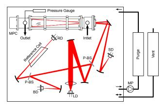
**Figure 1.** Optical system of the ISOWAT II spectrometer. LD: laser diode; P-BS: pellicle-beam splitter; MPC: multipass cell; SD: sample detector; RD: reference detector; BD: background detector; MP: miniature pump.
