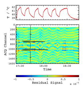
**Figure 5.** (a) Temperature recording of the mount of the  $f = 25.4 \,\mathrm{mm}$  collection lens. (b) Array of spectral residuals recorded in the laboratory while repeatedly modulating the temperature of the  $f = 25.4 \,\mathrm{mm}$  collection lens. The color code represents the residual amplitude scaled to optical density. The black trace depicts a second-harmonic spectrum recorded at 1 s integration time.
