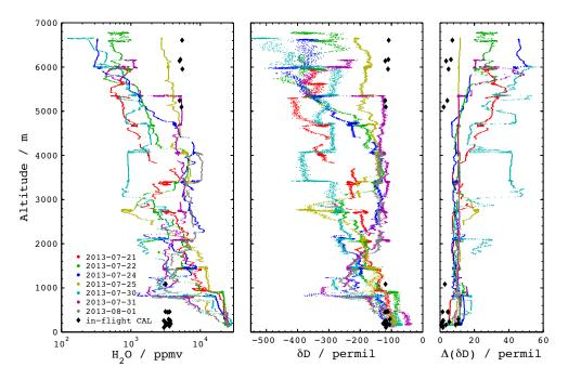
Figure 9. Vertical profiles of  $H_2O$  (left),  $\delta D$  (center), and instrumental absolute uncertainty (right) of all flight days evaluated at 1 Hz. For better clarity we show here only data with aircraft descending. Black symbols denote the respective quantities of the inflight calibration-gas measurements.
