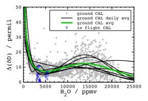
**Figure 4.** Uncertainty analysis for all flight days. Grey symbols: deviation of individual 1 Hz calibration measurements from calibration standard; black lines: daily fit of  $\Delta(\delta D)$  (Eq. 2); green line: campaign average of  $\Delta(\delta D)$ . Inflight calibration-gas measurements are depicted as the difference to the daily mean (absolute value) by the blue symbols.
