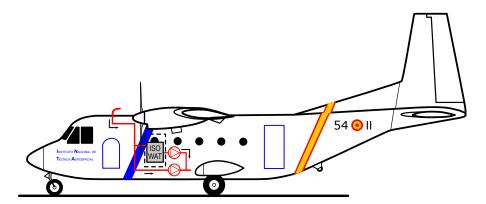
**Figure 7.** CASA C-212 aircraft of Instituto Nacional de Técnica Aerospacial (INTA). The rear-facing ambient air inlet was located on top of the fuselage. The inlet line was flushed at a high flow using a membrane pump. ISOWAT was mounted in the foremost position of the aircraft and was equipped with a second pump to establish the gas flow through the instrument.
