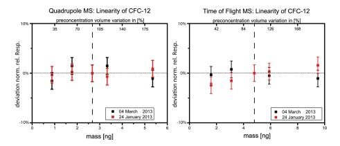
**Figure 7.** Same figure as Fig. 6 for the substance CFC-12 (CF<sub>2</sub>Cl<sup>+</sup> fragment).
