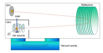
**Figure 2.** Scheme for the direct ion extraction of the Bench TOF-dx direct extraction (five technologies GmbH, G. Horner and P. Schanen, personal communication, 2014). The red dotted line represents a typical ion path.
