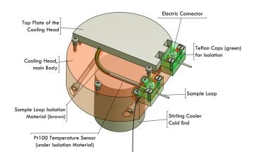
**Figure 1.** Schematic of the cooling head. The aluminium cylinder which contains the sample loop is placed on top of the Stirling cooler's cold end. Electric connectors are located at each end of the sample loop for resistive heating.
