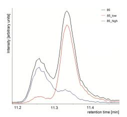
**Figure 5.** A chromatogram of an unidentified hydrocarbon peak (smaller one) eluting slightly earlier than the higher Trichloromethane peak. The nominal mass 85 u (black) shows a double peak. By choosing the lower mass range (84.7 u to 85.0 u; red) a lower signal for the unidentified hydrocarbon peak is observed, and by choosing the higher mass range (85.0 u to 85.3 u, blue) a lower signal for the Trichloromethane peak is observed.
