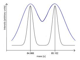
**Figure 3.** Schematic display of two different mass resolutions (blue and black curves). Two signals on masses 84.966 and 85.102 u with equal intensities demonstrate the mass separation with R=600 (blue curve) and R=3700 (black curve). Assuming Gaussian peak shapes for the signals, R=3700 separates both peak by  $8\sigma$  (quantitative separation) and R=600 separates them by only  $2\sigma$  (qualitative separation).
