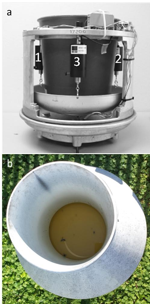
**Figure 1.** Photographs of the Geonor T200B gauge (a) interior out-fitted with redundant sensors and (b) looking through the gauge opening to the exposed interior reservoir.
