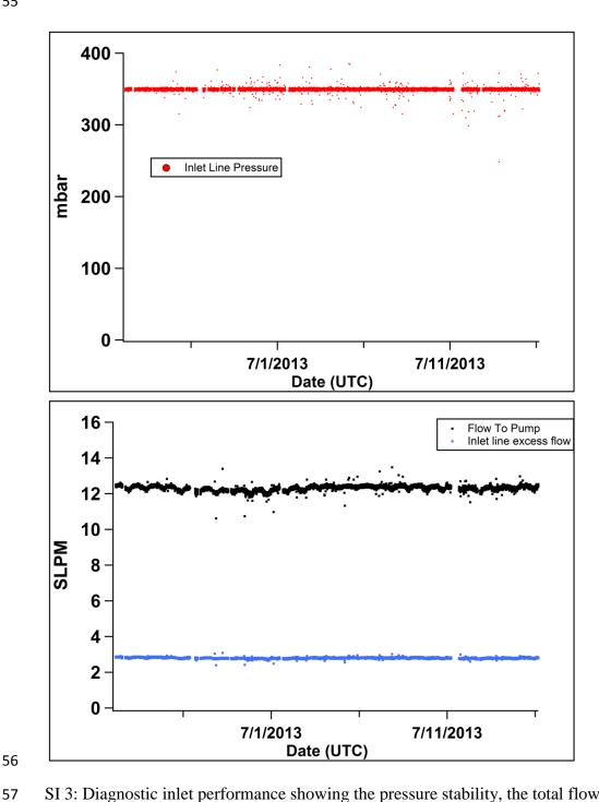
SI 3: Diagnostic inlet performance showing the pressure stability, the total flow through the gas sampling line, and the total flow to the pump during SOAS.
