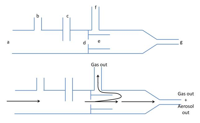
SI 2: Glass inlet design (a) aerosol and gas inlet; (b) zero air overflow port; (c) calibration port (not used in this study); (d) critical orifice; (e) glass particle skimmer and flow director; (f) gas sampling port at reduced pressure; (g) bypass line at reduced pressure
