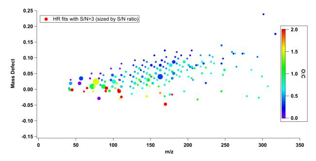
SI 5: Mass defect enhancement plot showing all species with S/N>3 and colored by oxygen:carbon ratio as determined from the HR ion fits.
