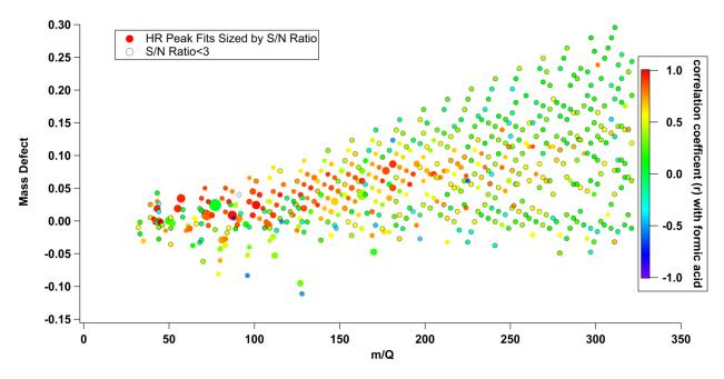
SI 4: Mass defect plot showing all HR ion fits. Each ion fit is colored by the correlation coefficient with formic acid and sized by S/N ratio. Ions with a S/N<3 are marked with a black circle outline.
