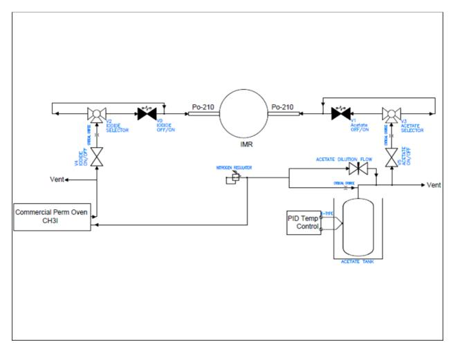
SI 1: Schematic diagram showing the setup for reagent switching with selectable flow path for automatic switching driven by solenoid valves or manual control.
