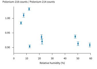
**Figure 4.** Ratio of polonium–218 to –214 counts (related to the recoil probability,  $p_r$ ) during pulse injection tests as a function of the average relative humidity within the detector for the first hour since pulse injection. The Bayesian deconvolution approach (Sect. 3.3) was used to fit the model to observations by specifying a known ambient radon concentration. The markers show mean  $\pm$  one standard deviation.
