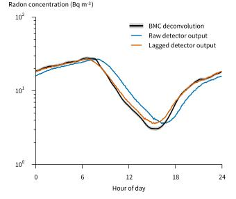
**Figure 10.** Composite diurnal cycle from the Richmond 1500 L detector during 2 weeks of consecutive stable nights and clear-sky days. BMC deconvolution means the Bayesian Monte Carlo deconvolution method from Sect. 3.3 and the 16th—84th percentile range is shaded grey. A lag correction of 72 minutes maximises the correlation between the lagged detector output and the deconvolved output. See Chambers et al. (2015b) for site details.
