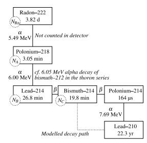
**Figure 2.** The decay series of radon and its immediate progeny, an extract from the uranium–238 series. The figure shows the energy of alpha decays, and nomenclature used to identify species abundances:  $N_{\text{Rn}}$ ,  $N_A$ ,  $N_B$ , and  $N_C$ .
