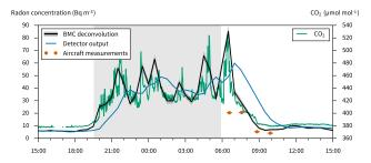
**Figure 7.** Field observations from a calm and clear night on the 5th–6th of November 2011. The wind speed was  $\leq 1 \text{ m s}^{-1}$  at 2 m a.g.l. for most of the night. Aircraft measurements were made 36–41 m a.g.l. over 6 km flight segments. Night-time is shaded grey, as is the 16th–84th percentile range about the reconstructed time series.
