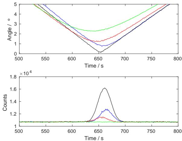
**Figure 2.** Moon intrusion event in different deep-space views on 30 October 2015, with MHS on MetOp-A; blue: DSV 1; black: DSV 2; red: DSV 3; green: DSV 4. Top: angle between Moon and space view. Bottom: space view count.
