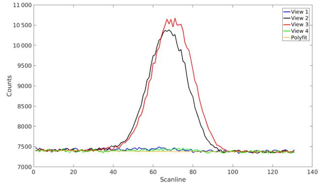
**Figure 4.** Moon intrusion event in different deep-space views on 17 July 2015 with MHS. The position of the Moon falls almost exactly between DSV 2 and 3 just so it affects the counts in all four positions. The orange line gives the number of counts in views 1 and 4 without any contribution from the Moon; it falls below the actually measured count levels from all four space views during the closest approach of the Moon.
