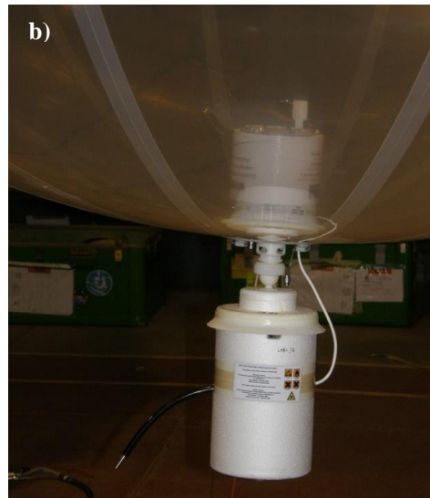
Figure 1. (a, left) The LOAC gondola with a Meteomdem Company sonde for flight under meteorological balloons; (b, right) the LOAC gondola below a low troposphere drifting balloon.
