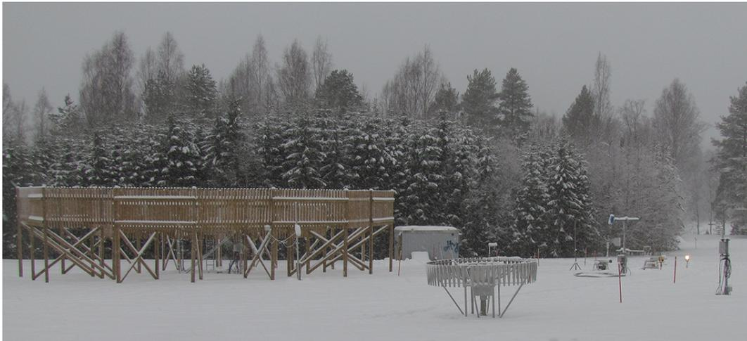
**Figure 1.** Snow precipitation instruments on the measurement field in Hyytiälä. The Pluvio<sup>2</sup> 200 is inside the wind protection on a platform and the PIP lamp can be seen at right on the ground. The view of the picture is to southwest and the distance from the platform to the treeline behind is approximately 20 m.
