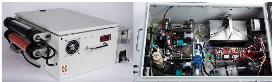
**Figure 2.** The exterior (a) and interior (b) of the new OPROSI. All components shown are attached and integrated into, or onto, a portable box (60 × 50 × 25 cm) to allow easier deployment for field studies.
