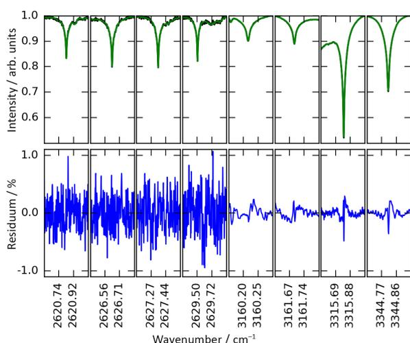
**Figure 1.** An example fit of the measured (black) with the calculated (green) spectrum and their residuals (blue) for the various microwindows used. Note the different signal-to-noise ratio due to different instrument setup (see Sect. 2.2).
