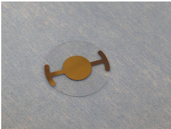
Figure 1. Piezoelectric crystal microbalance: quartz crystal (transparent plate) and gold electrode in the centre. On the right side and left side are the contact points for the proximity electronics.
