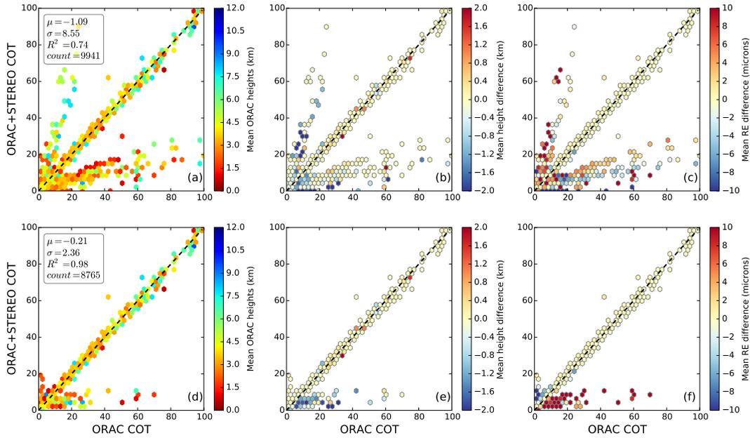
**Figure 10.** Joint histograms of COT as retrieved by ORAC and by ORAC+stereo. Plots (a–c) show the samples for all single-layer clouds over water (number of layers determined by CALIOP and open water determined by AMSR-E). Plots (d–f) show the subset of the sample where the ORAC and ORAC+stereo phases are in agreement.
