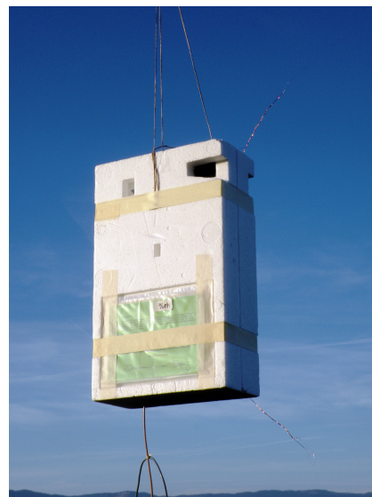
Figure 13. Meteolabor SRS-C34 radiosonde with original thermocouple temperature sensor fixed to thin wires that extend at a 45° angle upward (above right) and an additional thermocouple temperature sensor at a 45° angle downward (below right).
