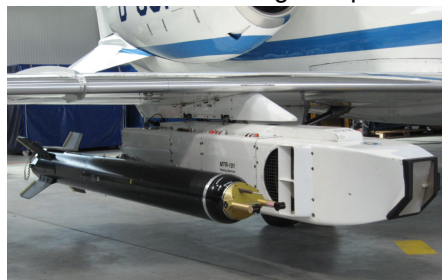
(b) AIRTOSS connected to the winch under the right wing of the aircraft.
