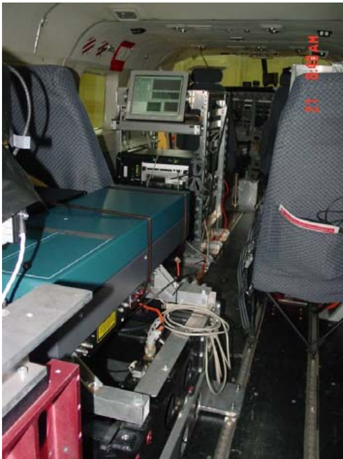
Fig. 1. TROPOLEX system installed on the DLR research aircraft Cessna Grand Caravan.
