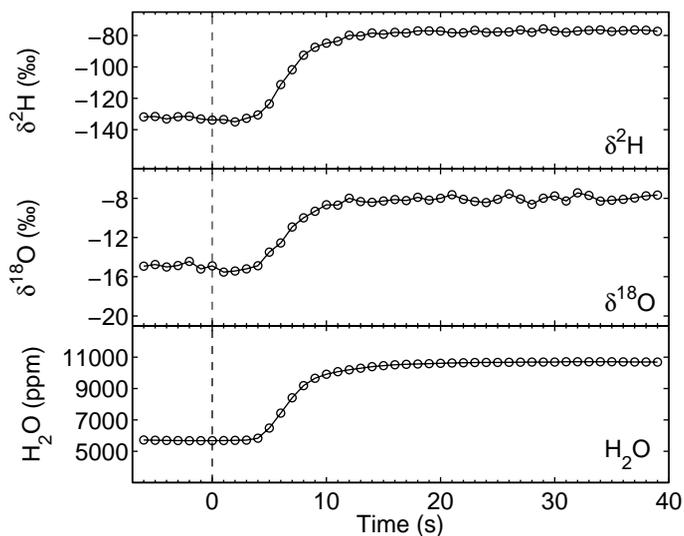
**Fig. 4.** Response time of a step change (at  $t=0$  s) when inlet air is switched from sample to calibration at a flow rate of  $800 \text{ mL min}^{-1}$  for  $\delta^2\text{H}$  (top),  $\delta^{18}\text{O}$  (middle) and  $\text{H}_2\text{O}$  (bottom). The time lag after the switch is  $\sim 4$  s and the time constant of the exponential change is  $\sim 3$  s.
