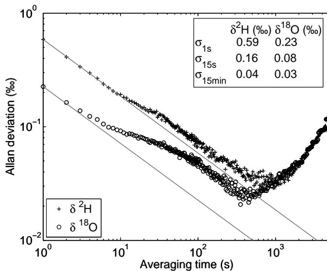
**Fig. 2.** Allan plots of  $\delta^2\text{H}$  (plus signs) and  $\delta^{18}\text{O}$  (circles) as a measurement of signal stability. The black lines show the theoretical slope for white noise. The upper insert shows Allan deviations (square root of the Allan variance) for different averaging times.
