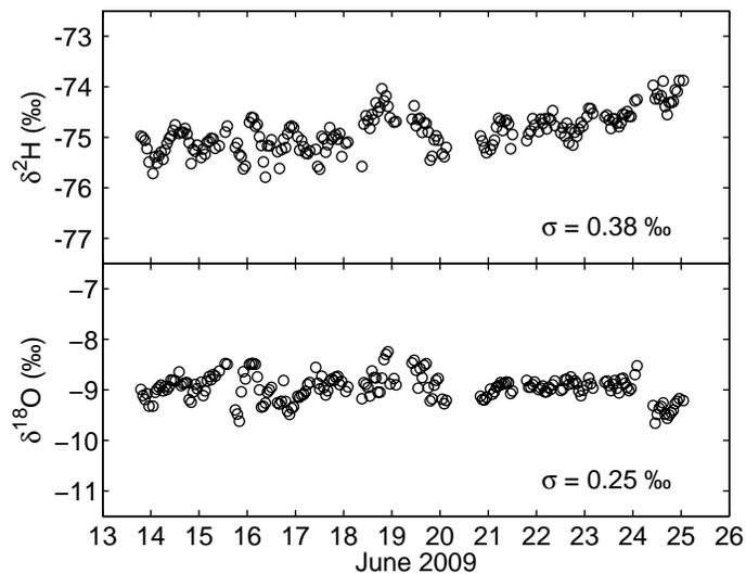
**Fig. 10.** Repeated analyses of a local water standard with our calibration system during 12 days. The standard deviation is 0.38‰ for  $\delta^2\text{H}$  and 0.25‰ for  $\delta^{18}\text{O}$ , respectively.
