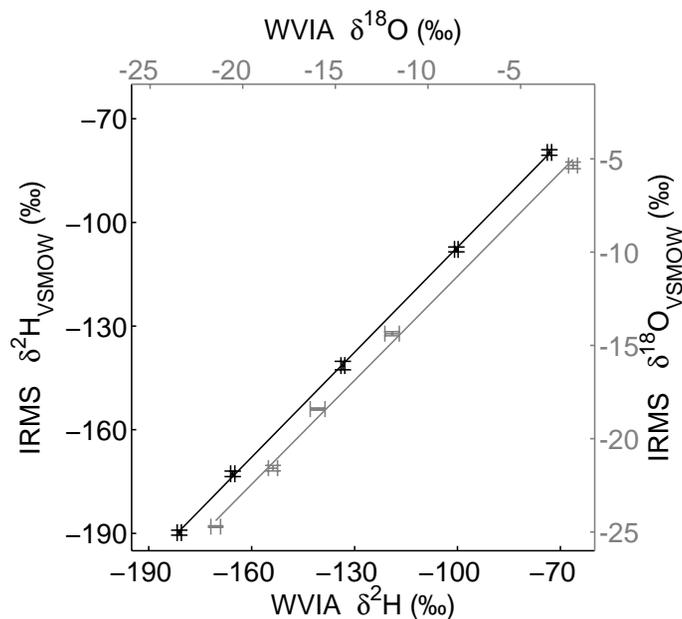
**Fig. 9.** Calibration of  $\delta^2\text{H}$  (black) and  $\delta^{18}\text{O}$  (grey) with different water standards. Weighted least squares fit through the data results in  $\delta^2\text{H}_{\text{IRMS}} = (1.013 \pm 0.011) \delta^2\text{H}_{\text{WWIA}} - (5.82 \pm 1.53)$  and  $\delta^{18}\text{O}_{\text{IRMS}} = (1.007 \pm 0.019) \delta^{18}\text{O}_{\text{WWIA}} - (2.92 \pm 0.32)$  (solid lines),  $R^2 > 0.99$ .
