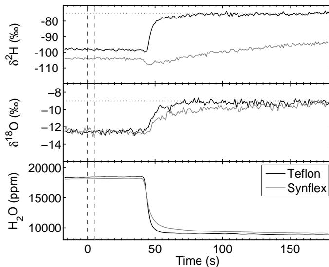
**Fig. 5.** Response time of a step change when inlet air is switched from sample to calibration and led to the WVIA through  $\sim 32$  m of Teflon tubing (black line) or  $\sim 27$  m of Synflex tubing (grey line), respectively, at a flow rate of  $450 \text{ mL min}^{-1}$ . The Synflex data are shifted by 5 s to account for the smaller time lag after the switch (dashed lines) due to the shorter tubing length. The dotted lines are the target values of the isotope ratios.
