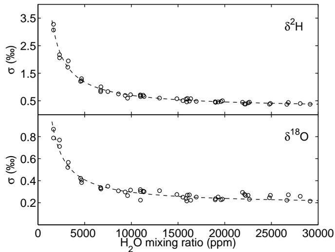
**Fig. 3.** Standard deviations of 1 s measurements of  $\delta^{2}\text{H}$  (top) and  $\delta^{18}\text{O}$  (bottom) as a function of  $\text{H}_2\text{O}$  mixing ratio. The dotted lines show  $1/x$ -fits.
