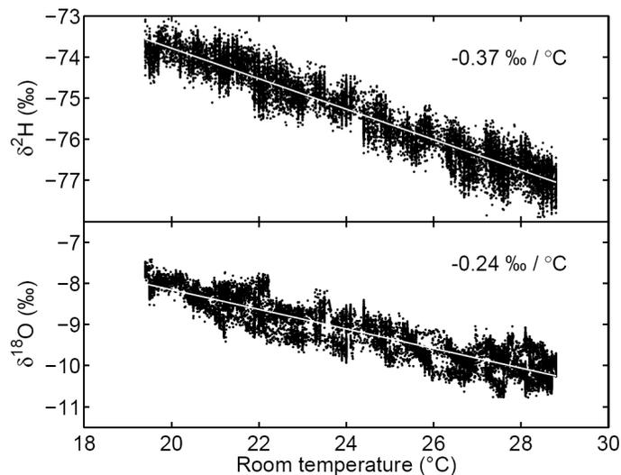
**Fig. 7.** Sensitivity to room temperature variations for  $\delta^2\text{H}$  (top) and  $\delta^{18}\text{O}$  (bottom). The dots are 10 s averaged data and the ordinary least squares fits yield slopes of  $-0.37\text{‰}/^\circ\text{C}$  ( $R^2=0.92$ ) and  $-0.24\text{‰}/^\circ\text{C}$  ( $R^2=0.82$ ) for  $\delta^2\text{H}$  and  $\delta^{18}\text{O}$ , respectively (white lines).
